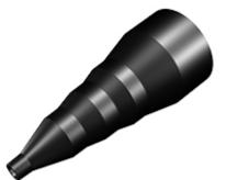
4" to 1" Adaptor is tapered from the 4" O.D. to the 1" O.D. Cut the adaptor at the desired diameter to fit to your machine port or smaller I.D. hose. Flat portions are at sizes of: 4", 3", 2-1/2" and 1" for hose to hose splices. Hose clamps are required.
